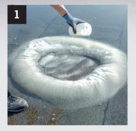
Sprinkle the granulate directly into the standing water around the work area. A gel forms. A solid dam, which reliably keeps back the water is formed within only 3–5 minutes. If necessary, sprinkle more granulate in the work area.
