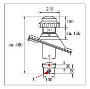
1. Can be extended to DN 125 by unscrewing the screws and removing the reducing adapter
