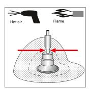
First shrink the heat-shrink sleeve evenly and completely onto the flange socket at the bottom.
