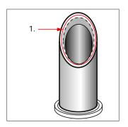
For increasing the DN 50 bushing, it is provided with a predetermined breaking point
